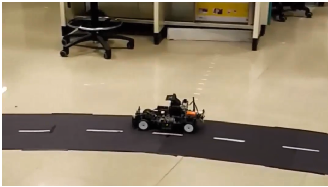
Fig. 5. Autonomous ground vehicle used for lane following tests without seeing the lane.
